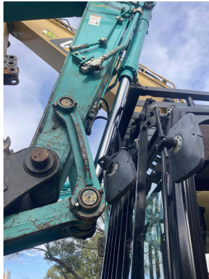
Image Comment(s): Another Machine cylinder resting against ROPS when first arrived on site
