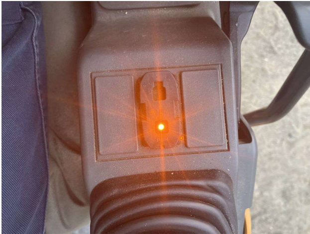
Image Comment(s): Rocker switches missing identification covers.
