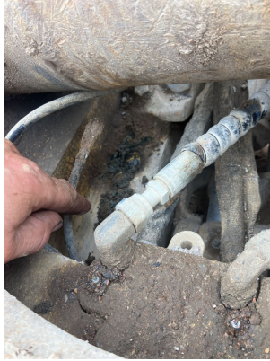
Image Comment(s): Coupler grease lines damaged.
