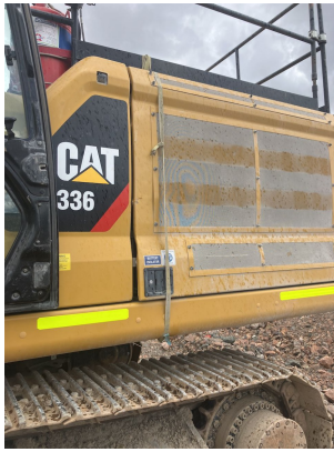
Image Comment(s): Left engine bay door damaged and latch not working.
