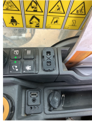
Image Comment(s): Switch cover missing.
