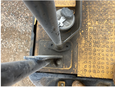
Image Comment(s): Handrail damage.
