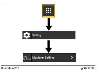
From the main screen, press the application menu button. In the Application menu, select "Setting" . Next, select "Machine Setting" .
