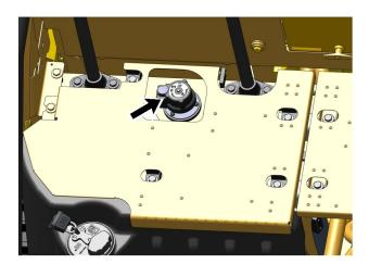
Hydraulic tank filler cap location
