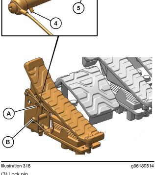
**Note:** To prevent lock pin (3) from being accidentally pulled out, insert pin (4) through notch (5) and turn lock pin (3) by 1/4 turn.
