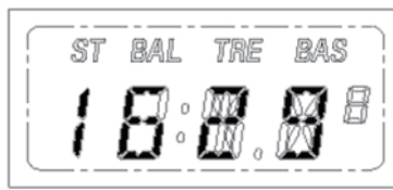
Frequency display (When AM is selected, "ST" pict always turns on)
