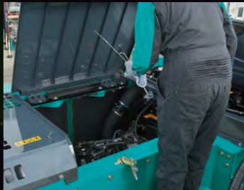
Engine maintenance A special lower access step near the engine simplifies maintenance.
