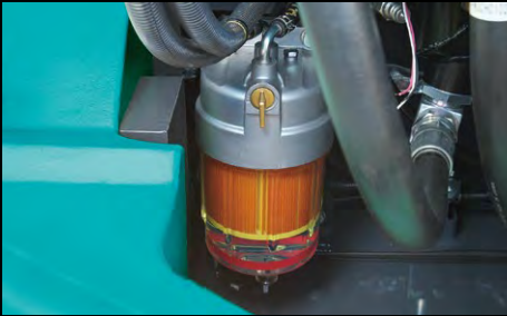
Enlarged fuel filter The enlarged fuel filter with built-in water separator maximises filtering performance.
