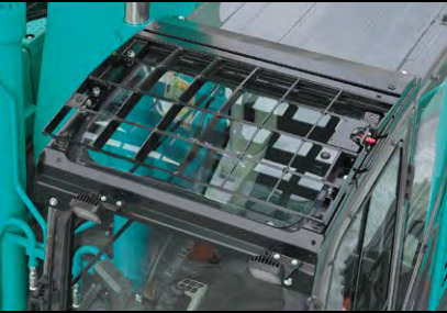
Standard FOPS overhead cab guard The standard FOPS guard can be tilted open for easy window cleaning. Meets standard FOPS, Top Guard Level II requirements. (ISO10262)
