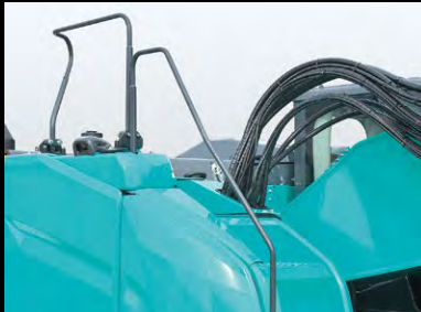
Handrail The handrail on the step side allows easy access to the maintenance port on the upper arm.
