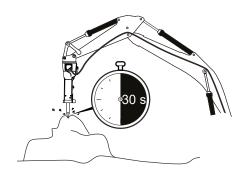
If the material fails to break, apply the tool to a new location.
