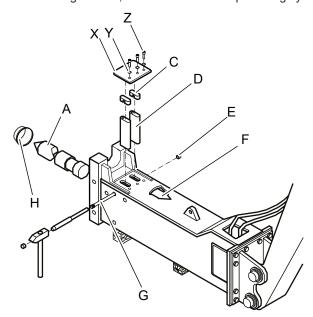
Wiper installed (only hydraulic breakers with DustProtector):
