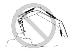
Slightly swing the hydraulic breaker to and fro when carrying out the hammer impacts, but never swing it through more than approx. 5°.
