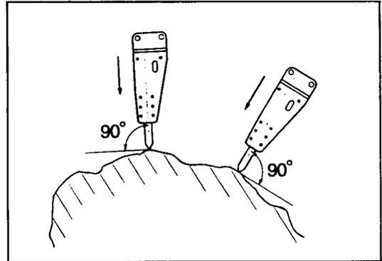
When operating the breaker, raise the chisel against the object and the front portion of the excavator about 5 cm from the ground.
