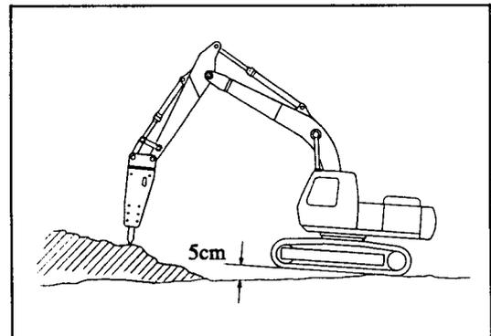
When breaking up an object which is large and hard, start where the rock can be easily broken.
