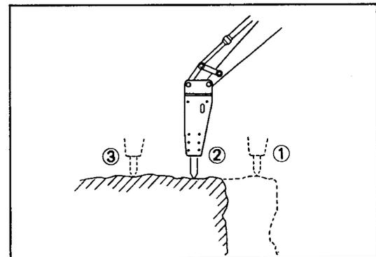
After striking against the same point continuously for 1 minute without the rock breaking, change to another area of the rock.
