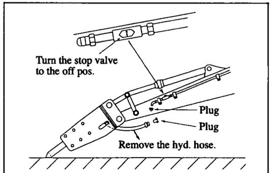
④ Remove the hyd. hose from the stop valve.
