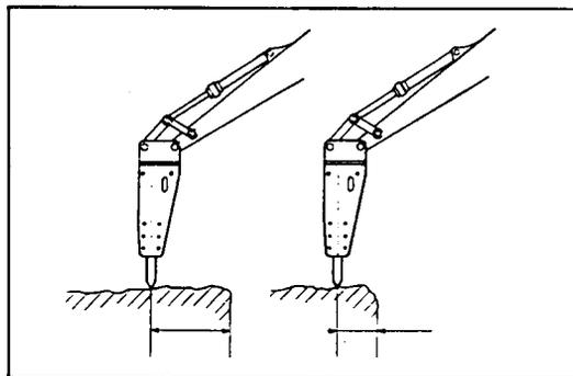
When the breaker is set to demolish an object, the impact angle changes slightly during operation. Constantly adjust the angle using the bucket cylinder of the excavator.
