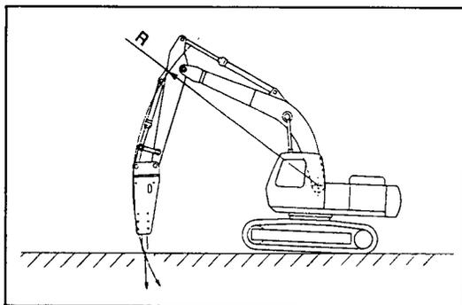
During impact, prevent blank blows by using the breaker properly.
