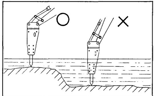
When using the breaker under water, refer to the instructions for underwater application on page 39 and 40.
