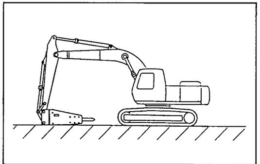
⑦ Operate the excavator and place the hydraulic breaker in a flat and stable place.
