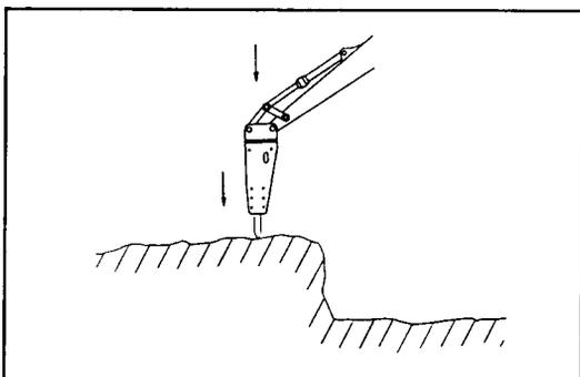
As soon as the material has broken, immediately remove your foot from the operating pedal to stop striking the material.
