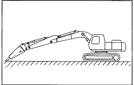
② Stop the excavator engine and remove the excess pressure in the hose.
