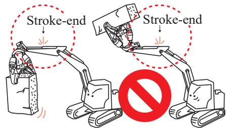
**⑦ Do not jack up the hydraulic excavator using the attachment**
