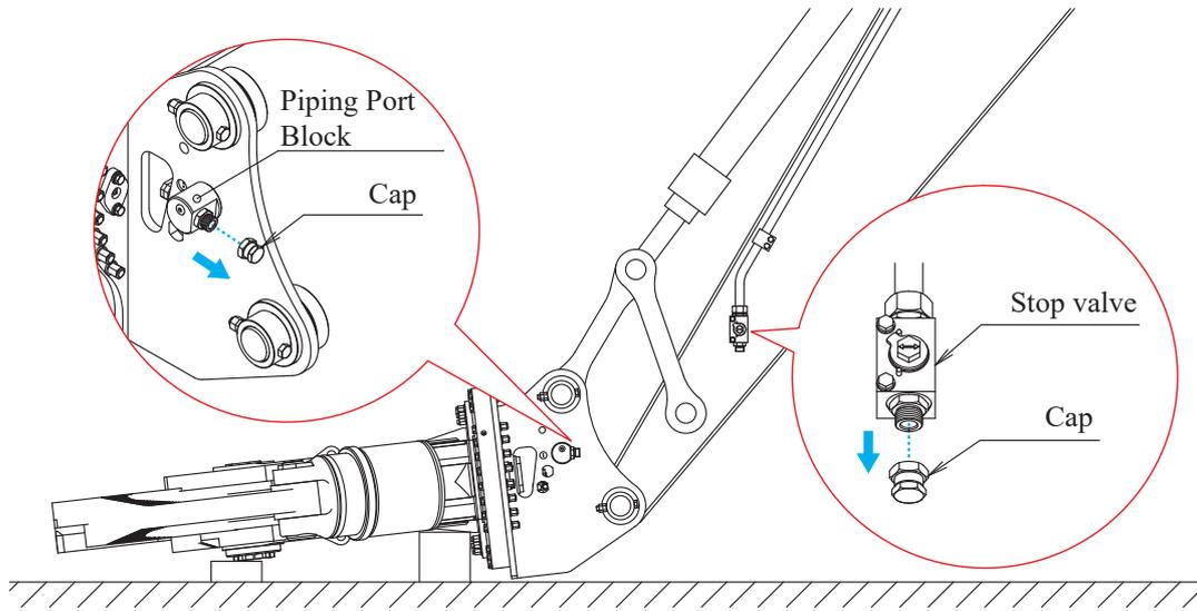
**6** Remove the hose plugs from both ends of the connection hydraulic hose, and then connect the attachment and hydraulic excavator while not bending the hydraulic hose. When connecting the hydraulic hose, make sure that no dirt, mud, or other foreign body gets in the hydraulic hose.
