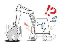
• When operating an attachment or working equipment (boom and arm), take sufficient care not to hit the excavator body.
