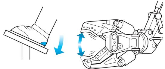
**2** With the jaw completely open, continue to step on the heel to start rotation.
