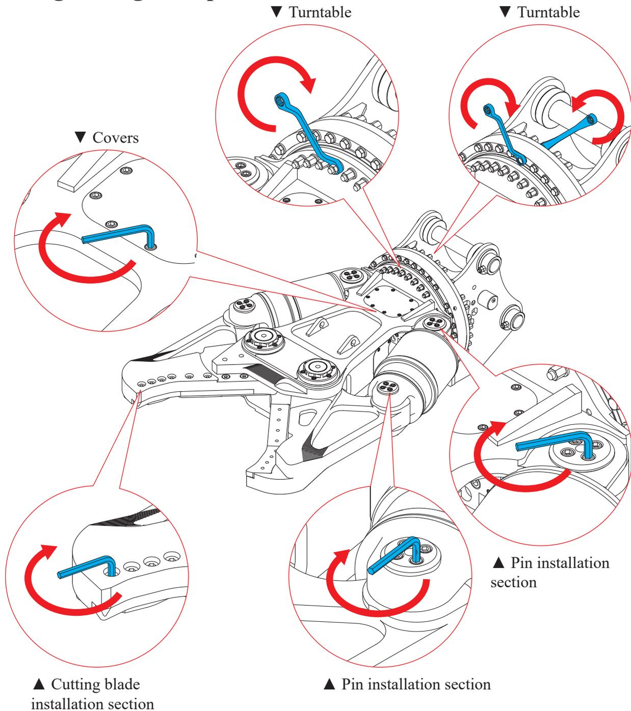
Always retighten using the prescribed torque. For the prescribed torque, see the standard torque table.
