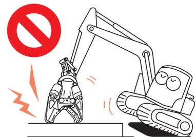
**⑧ Do not use the turning force of the hydraulic excavator to create an impact**
