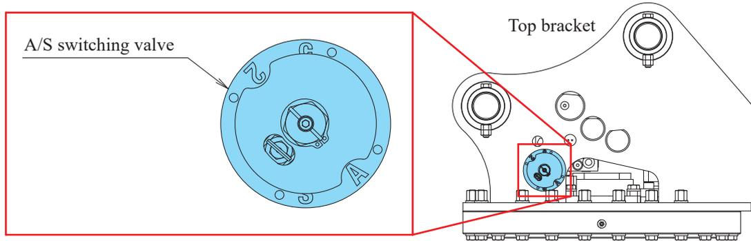
Turn the A/S switching valve to the indicated position for the mode to be used.
