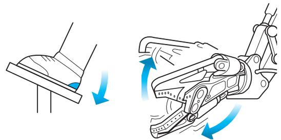
**3** Return the pedal to neutral at the desired crushing/cutting position to stop rotation.
