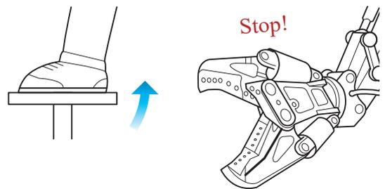
**4** Press down on the toe-end of the right pedal to crush or cut.
