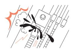
• Dirt, contamination, time-related deterioration, and other conditions of the hydraulic oil may cause problems for hydraulic equipment. Follow the inspection and maintenance rules for the hydraulic excavator and observe the exchange time for the filter (element) of the hydraulic circuit.
