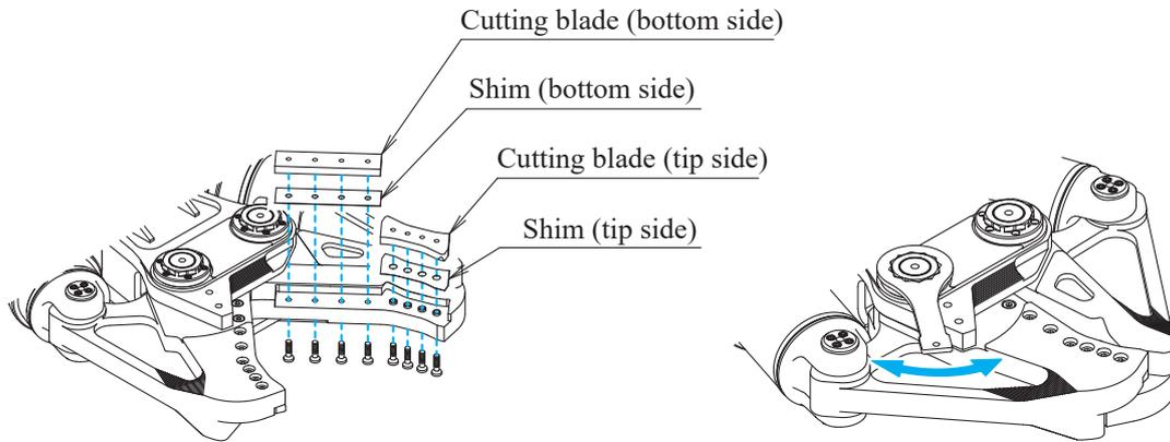
If the gap of the cutting blades exceeds **X mm** on both the bottom side and tip side, adjust the gap so that it is within **0.5 mm**.
