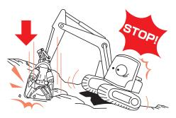
• Be careful that the hydraulic excavator does not tip over when working with heavy loads on sloping land. Furthermore, do not swivel the hydraulic excavator.
