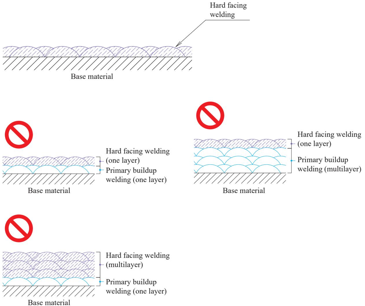
Use a welding rod of JIS Z 3251 DF3C or equivalent.
