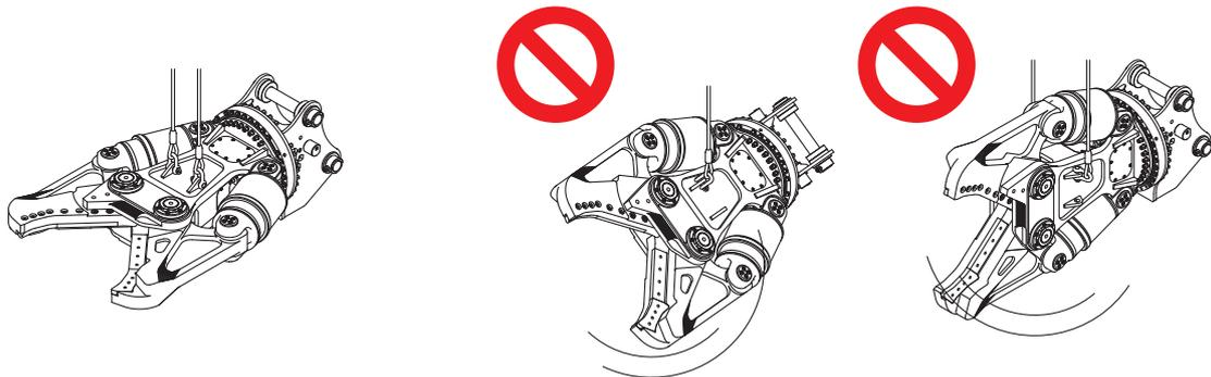
**2** After lifting the attachment a few centimeters from the ground, stop temporarily and wait for the attachment to stabilize before raising it up slowly.
