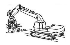
Don't have to strike down by the crusher. It can lead to the heavy damage to the crusher.
